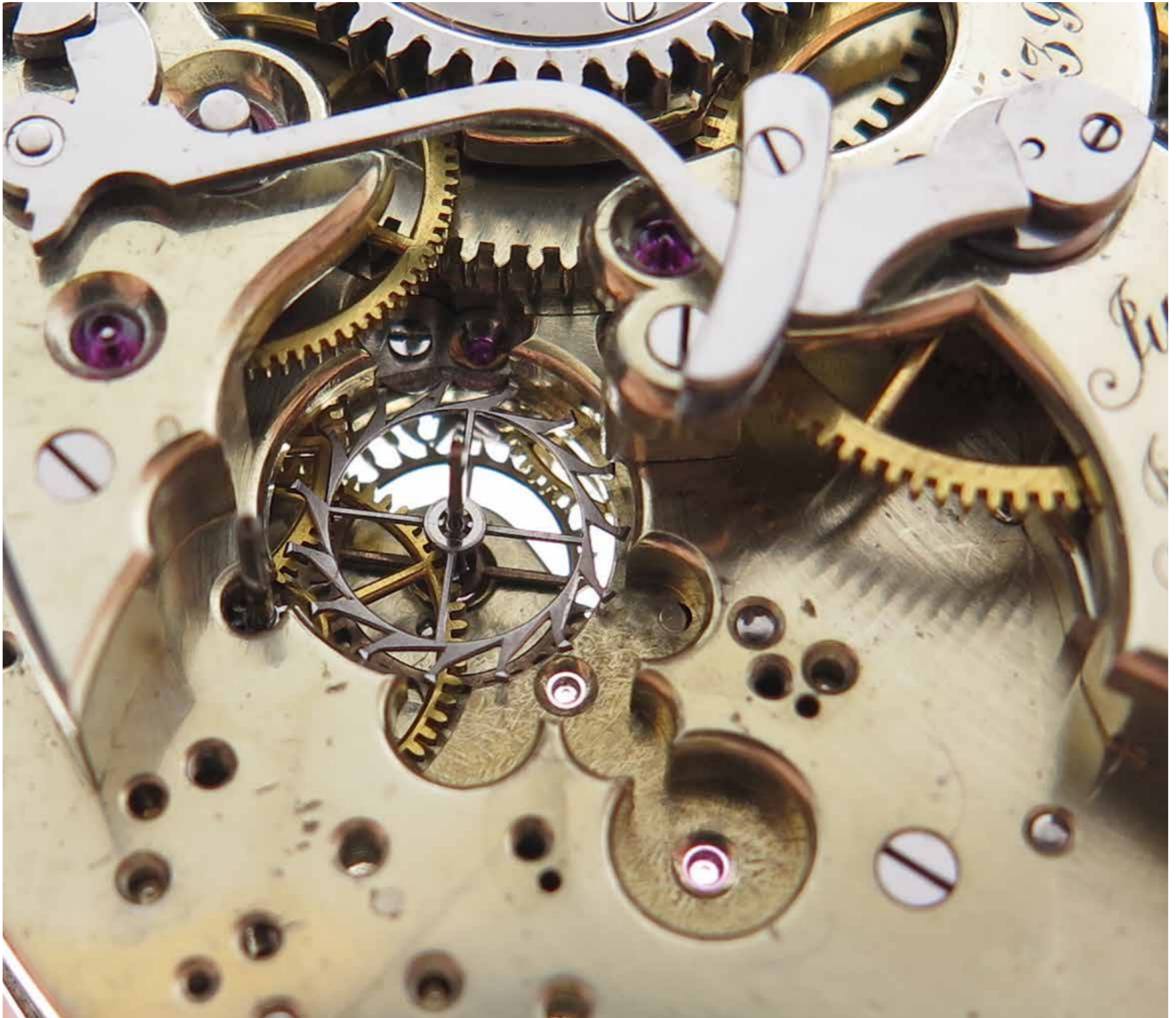
The escape wheel in place with the lever cock and balance removed.
